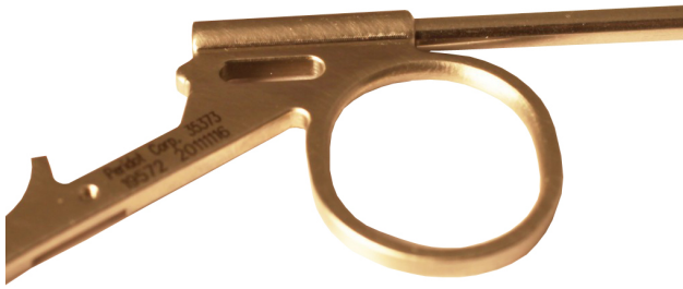
Custom machined and laser engraved forceps finger-pull laser welded to a 304 hypotube cannula
